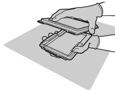
Figure 8: Sterile operator places the Hold Dish in the sterile field (gray rectangle)
